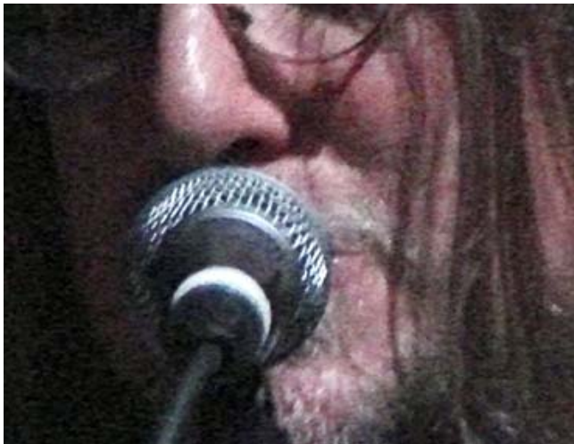
Figure 2-25 H5, ISO 800 Image, Brightened. Note the Loss of Color Saturation and Hair Detail to Noise Reduction
